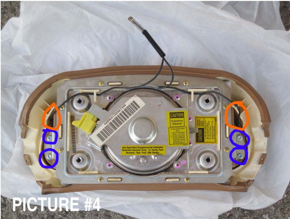
5. Place your new horn button in the housing, attach with the two screws you just removed and re-attach the one feed of the horn cable to the back end of the horn button.
