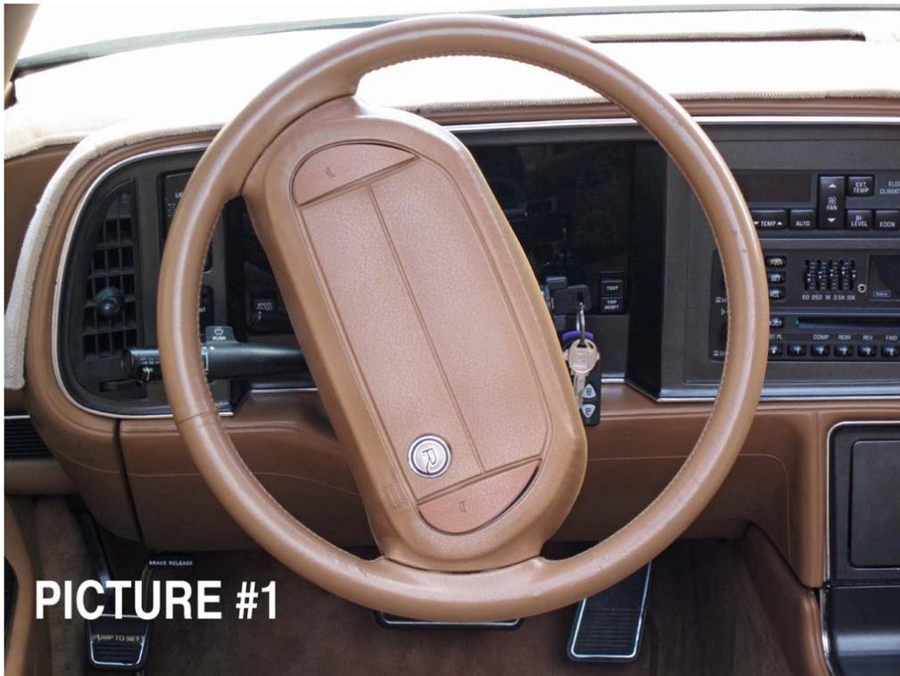
2. Turn off the engine, disconnecting the negative battery cable first and then the positive (to desensitize the airbag). Go have a cup of coffee and a danish. The air bag has an auxiliary power unit for deployment in case of an accident that causes the car battery not to work. It takes 30 minutes for that auxiliary capacitor to fully discharge (before handling the air bag) once the car battery has been disconnected.
